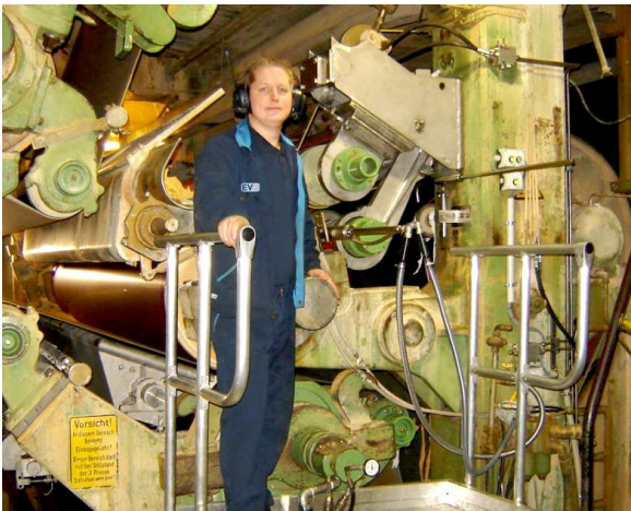
EV Project Manager, Mika Tähtinen was responsible for the PM6 press and single felted drying section modification with EVp, EVsp and EVsf web stabilizers.
